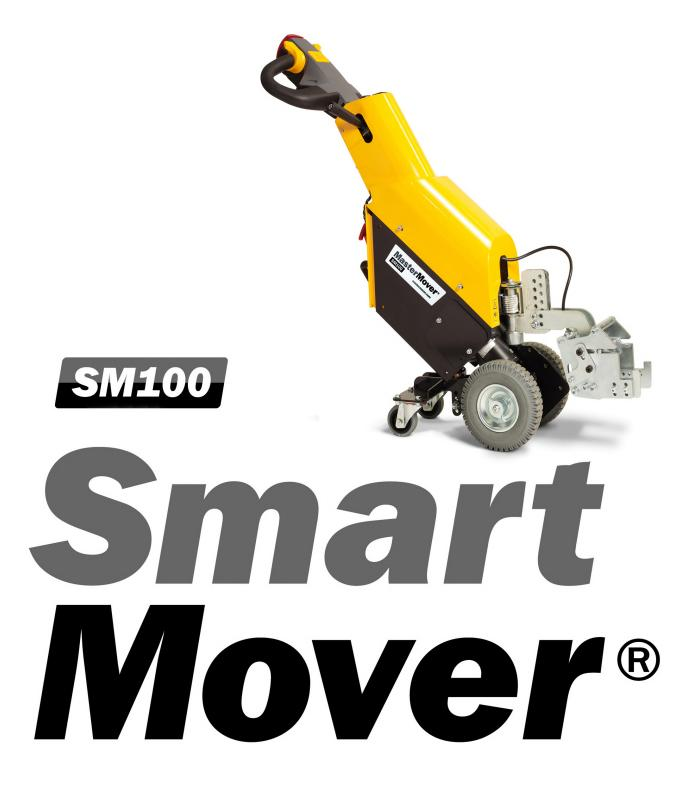
Battery Powered Tug | SmartMover® SM100 The SM100 is a battery powered tug that generates traction through a leveraged weight transfer system. A portion of the load weight is used to apply pressure on the optimally-sized wheels, allowing a single operator to easily move loads weighing up to 1,000 kg. A simple lever ensures a secure coupling to the load making the SM100 a safer alternative to manual handling of heavy wheeled loads, even on slopes or in congested areas.
