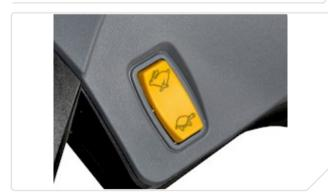
**Z41-00501**Option - flashing safety light and motion bleeper
