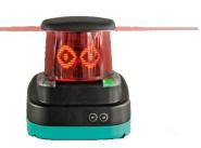
Navigation by magnetic tape tracking or free navigation by SLAM contour recognition, without the need for physical elements or markers, by triangulating the positions by the LIDAR sensor.
